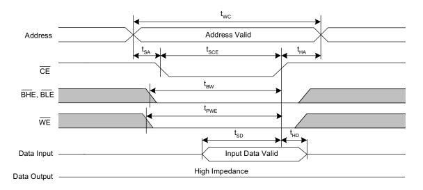
Figure 11. SRAM Write Cycle 3: BHE and BLE Controlled<sup>[5, 18, 19, 20, 21]</sup>
